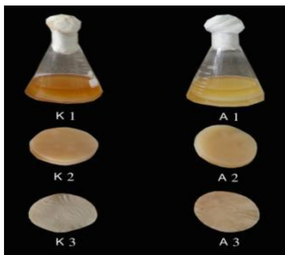
Photo. 1. BC pellicle of Komagataeibacter saccharivorans PE 5 and Acetobacter xylinum ATCC 10245 formed under optimized conditions, (K1,A1), fresh pellicle (K2,A2) and paper sheet (K3,A3)
